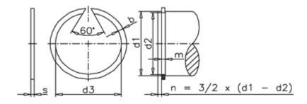
d3 = 92.0 Description = SW 95 FN kN = 49.20 FR kN = 61.80 m min = 2.7
